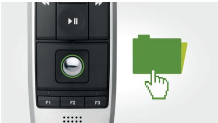
The Philips SpeechMike Air offers an integrated trackball that allows the user to easily navigate through documents and files without using a mouse.
