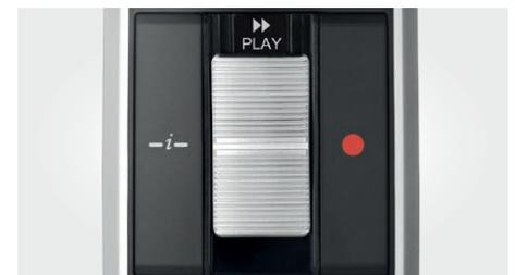
Slide-switch operation (fast forward, record/play, stop, fast rewind)
